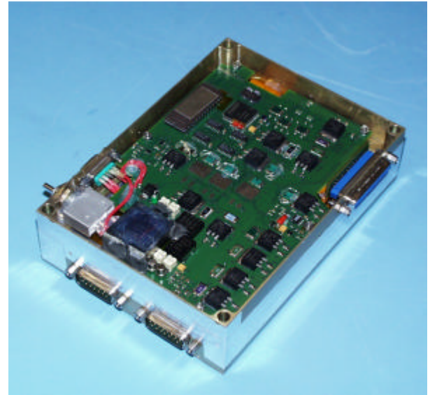
Fig. 7: Fully assembled SNAP-1 Power System in final configuration.
